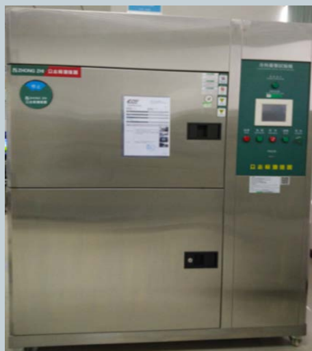
Thermal cycling tester
